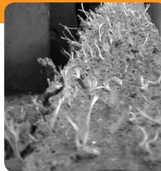
ASTM C1550 Panel Section at Failure— Macro-Synthetic Fibre
