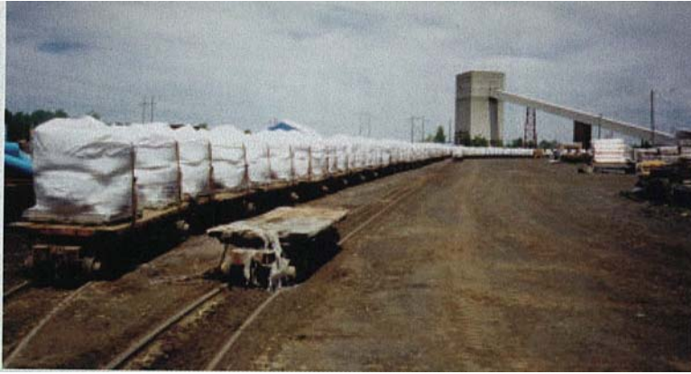
Shipment of prepackaged Shotcrete in 2205 lb (1 metric tonne) bags To an underground mine
