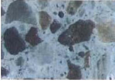
Fig 2: Non air-entrained shotcrete microstructure spacing factor: 0.016 in, (415 \mu\text{m} ) (60x magnification)
