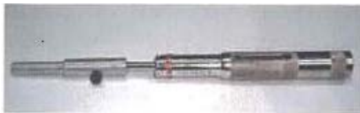
Fig 7: Portable penetrometer measuring plastic dry-mix shotcrete consistency.
