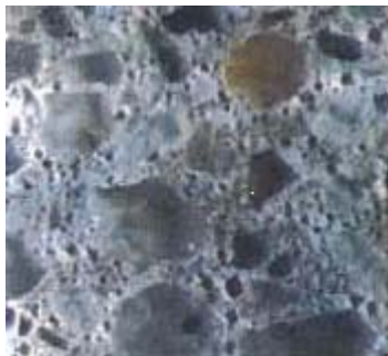
Fig. 1: Air-entrained Shotcrete microstructure; spacing factor: 0.004 in. (101 µm) 60x magnification).
