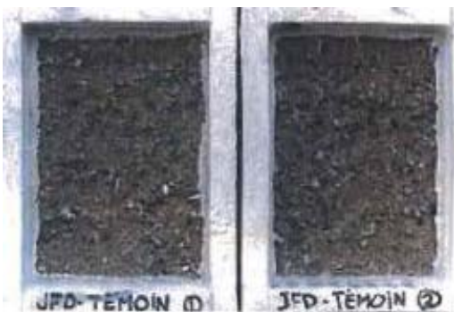
Fig 4: Resistance to deicing salt scaling-non air entrained; surface loss 1.8 lb/ft 2 (8.81 kg/m 2 )
