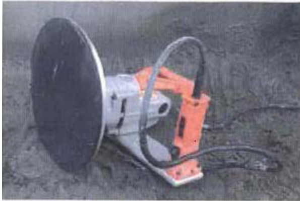
Fig 8: Mechanical spinning trowel with a high-density rubber disk
