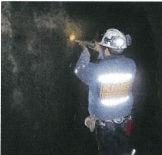
Fig. 3: Underground Schmidt Hammer Testing
